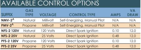
^ 35 ft. wire and millivolt thermostat are included with each NMV-2/PMV-2. Millivolt controls utilize a standing pilot flame for ignition therefore should not be used in windy environments. NFS-2/PFS-2 controls utilize potted circuit boards for protection in high moisture environments.
